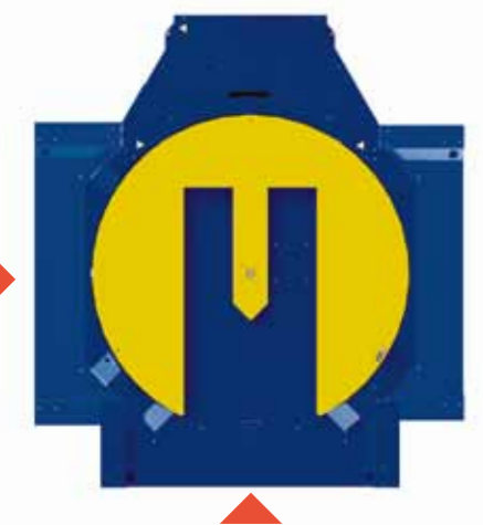
Horseshoe turntable with 3 in feed
